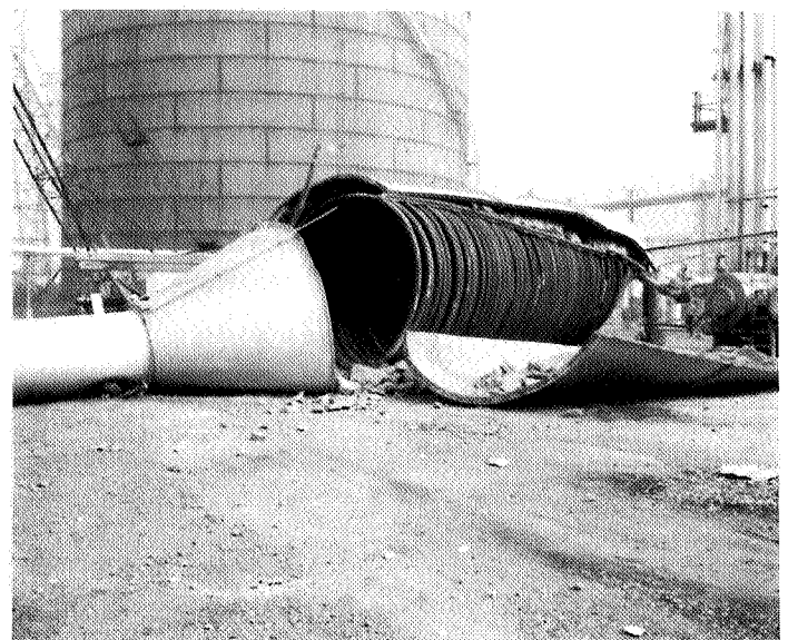
Figure 4. Photo of heater after the explosion.
